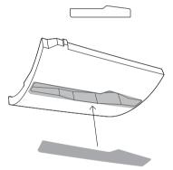
Alternatively, install the 3D printed hook well panel instead of kit part B86 (as per instructions step 12).
